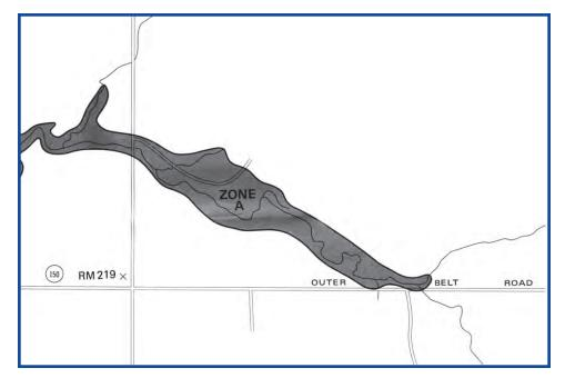
Topographic maps can be used to estimate the Base Flood Elevation.
