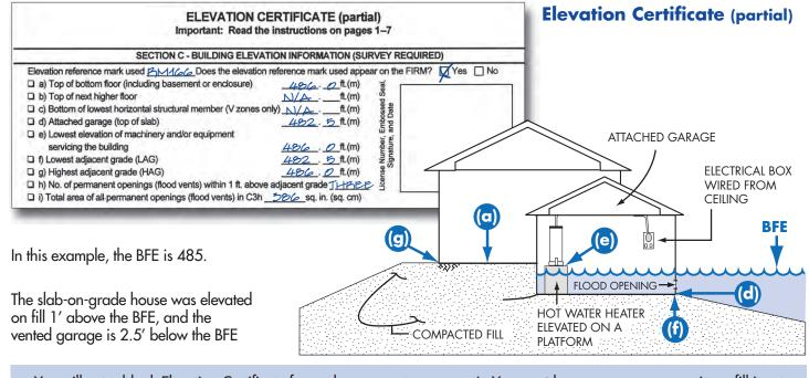
You will get a blank Elevation Certificate form when you get your permit. You **must** have a surveyor or engineer fill it out and seal it. The Elevation Certificate includes diagrams for eight buildings types. Several points must be surveyed.
